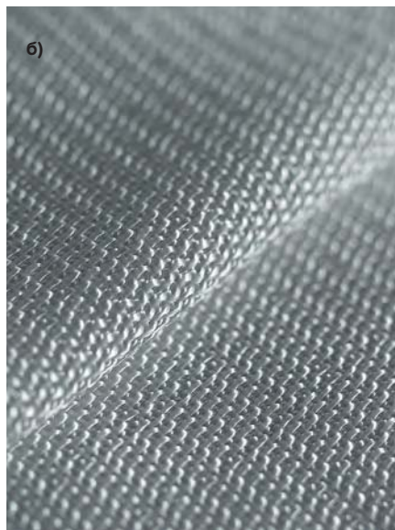
Fig. 3 TGF filter fabric, Ref. No.: а – traditional – series of Ref.No. 2V01, TFG-1 SG-1; б – upgraded – Ref.No. RF-3-13C15
