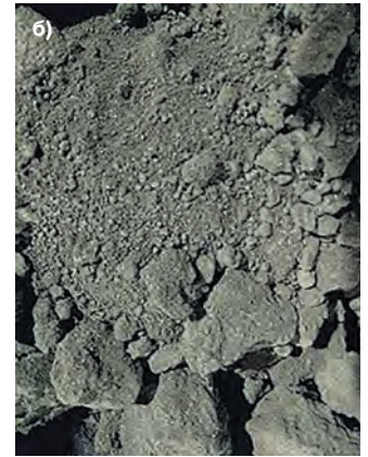
Fig. 9 Sample of the cake taken from the hog box mass: а – before drying; б – after drying
