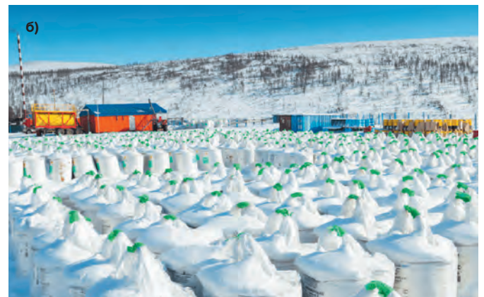
Fig. 1 Examples of projects completed by AZOTTECH LLC: а – PolyusVerninskoye, Bodaybo. Construction of a modular plant for preparation of emulsion explosives with the design capacity of 20,000 per year. Supply of explosives with borehole charging services using three own-made mixing and charging machines б – Pavlik Gold Mining Company (Arlan Investment Company), Magadan. Construction of a modular plant for preparation of emulsion explosives with the Berezit® emulsion explosive borehole charging services
