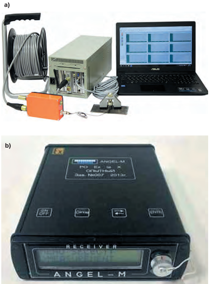
Fig. 1 (a) Acoustic emission complex A-Line DDM-1 (b) ANGEL-M device for EMR registration (developed by VNIMI)
