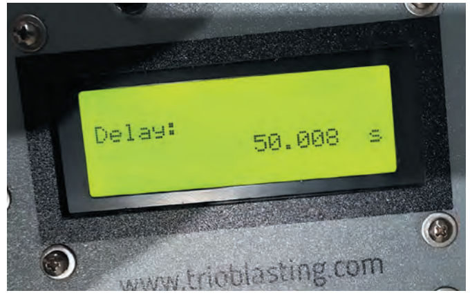
Fig. 3 Measuring the accuracy of electronic detonators
