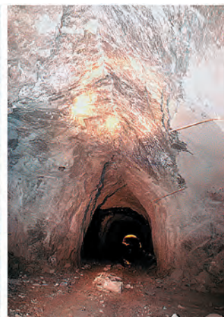
Fig. 8 Changes in the mine cross-sections as the result of dynamic manifestations of rock pressure
