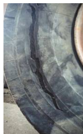
Fig. 3. amaged LHD tire
