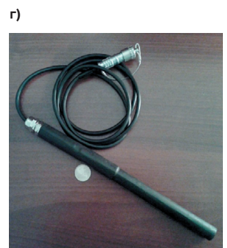
Fig. 6 External view of the ANGEL-M receiver (a), transmitting (б) and receiving (в) aerials and the KD35 acoustic sensor (г)
