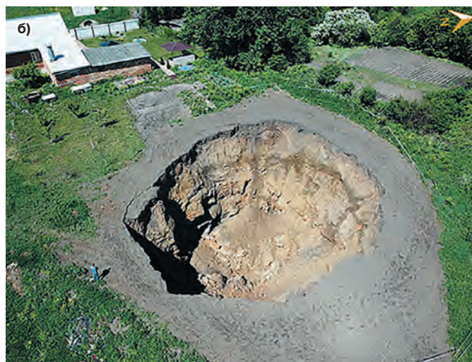
Fig. 3 UAV aerial photos of the karst sinkhole in the Dedilovo village (1) on May 18, 2019, in panoramic view (A) and at close range (B). Legend: straight white dashed lines connect the five karst sinkholes (1, 2, 3 and 2, 4 and 5)
