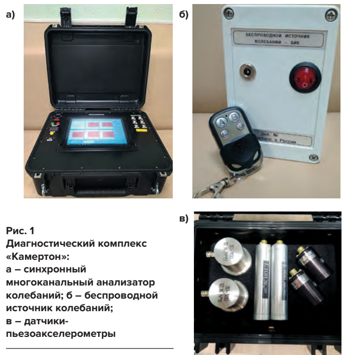
Fig. 1 The Kamerton diagnostic complex: a – synchronous multichannel oscillation analyzer; б – wireless oscillation source; в – piezoaccelerometer sensors
