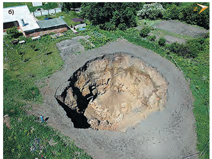
Fig. 3 UAV aerial photos of the karst sinkhole in the Dedilovo village (1) on May 18, 2019, in panoramic view (A) and at close range (B). Legend: straight white dashed lines connect the five karst sinkholes (1, 2, 3 and 2, 4 and 5)
