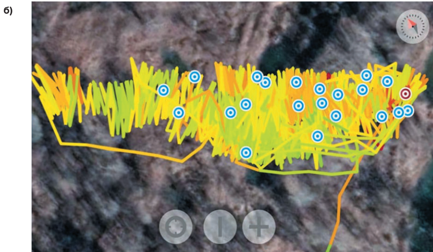
Fig. 1 An example of a bulldozer motion diagram: а – manually drawn based on the results of timing on 04.03.2025; б – using a geotracker based on the results of timing on 08.04.2025
