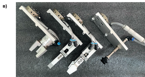
Fig. 6 A laboratory training cell: а – laboratory and technical complex; б – interactive control and programming panel for the manipulator; в – grippers for simulating technological processes
