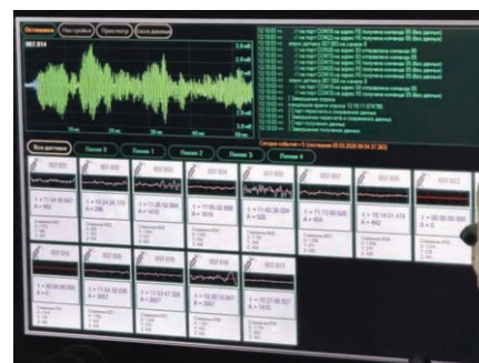
Fig. 6 Registration of dynamic manifestations of rock pressure using the ASKSM sensors in-situ
