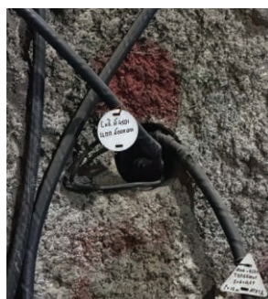
Fig. 6 Registration of dynamic manifestations of rock pressure using the ASKSM sensors in-situ
