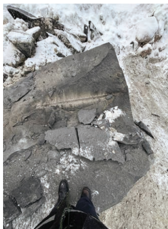
Fig. 1 An oversized rock split open using a composition with aluminum additive
