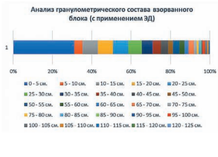
Fig. 2 Images of the rock mass and particle size distribution analysis of blasted block No. 1-2 when using electronic detonators
