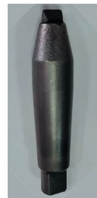
Fig. 1 Geometric parameters and a general view of the RS-14 commercial tangential non-rotating pick
